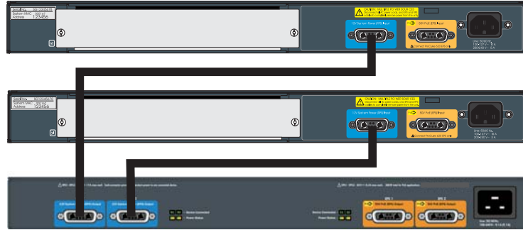
Figure 2-13. Connecting RPS to 2, 24 port switches.
